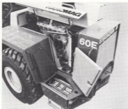
▲ Maintenance points are clearly and easily accessible.
