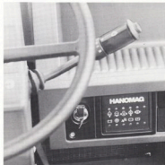
▲ "Centronic" — central electronic checking, warning and safety system
