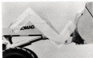
▲ Force reversal of the cross-over linkage during the work stroke of the piston
