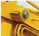
Bucket level indicator is within your line-of-sight. Nearby automatic return-to-dig switch is well-protected, yet easily accessible. Hydraulic self-leveling and float are also standard.
