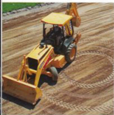
A 50-degree turning angle gives the 310E a tight 11-foot 9-inch turning radius for easy moves in close quarters.
