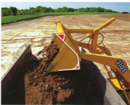
Torque tube spilloose construction (in red) prevents twisting and resists bending. C-shape backwall empties easily and sheds sticky materials.
