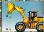
Dump clearance on the 744H MH is 10 feet 6 inches – higher than both the standard 744H (10 feet) and the 744E (9 feet 10 inches).
