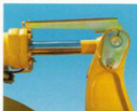
The return-to-level option brings the boom and bucket back into position, ready to get right into the next cycle.
