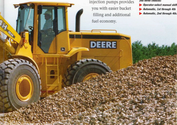
SMART-SHIFT technology delivers smoother shifts with less delay under all load conditions. The automatic shift feature gives you three choices:
